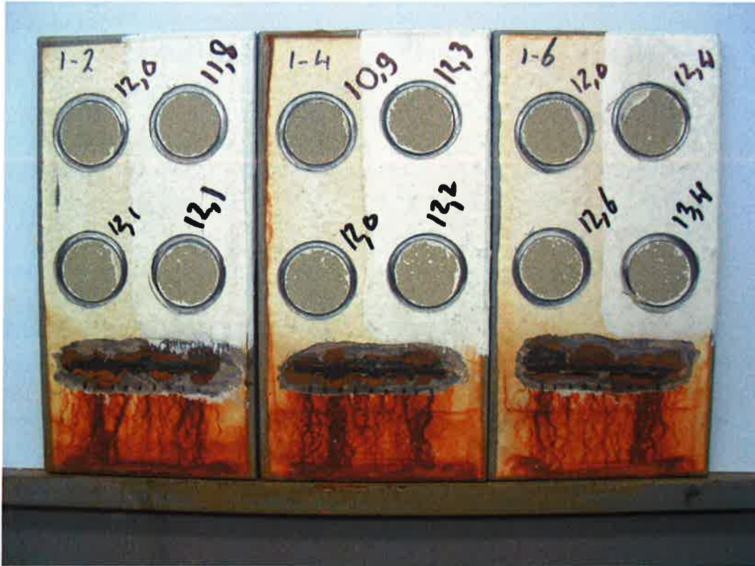
Photo 1. Cyclic ageing test, panels 2, 4 and 6.
