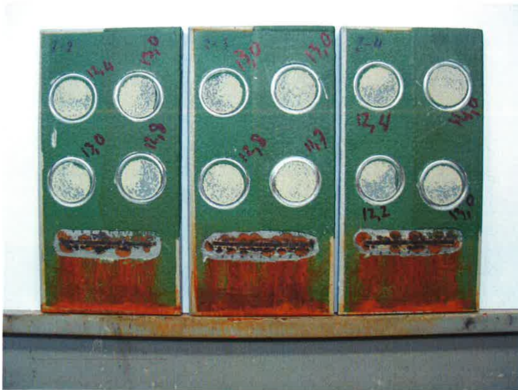
Photo 1. Cyclic ageing test, panels 2, 3 and 4.
