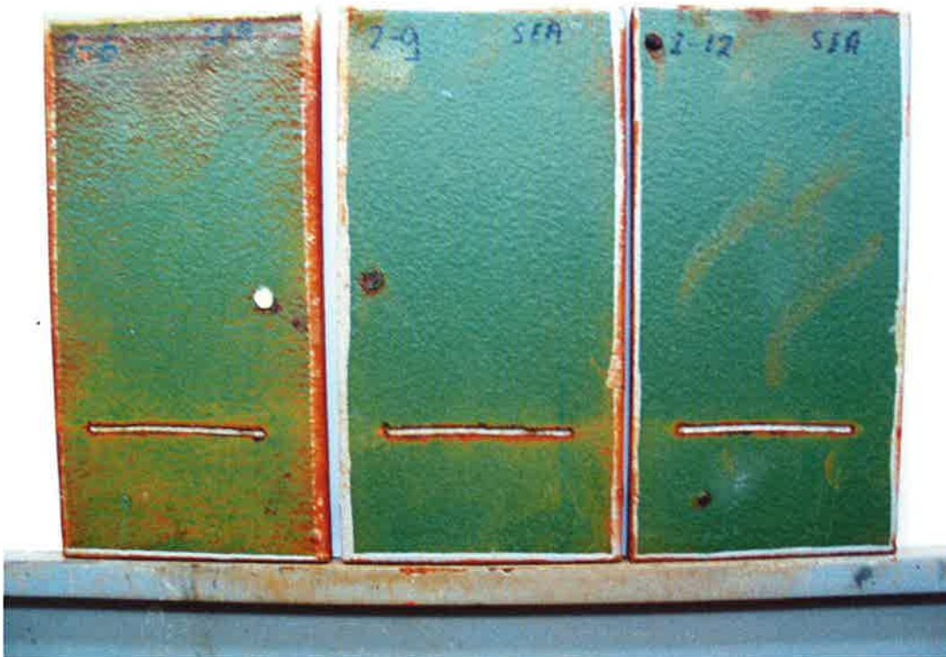
Photo 2. Seawater immersion test, panels 6, 9 and 12
