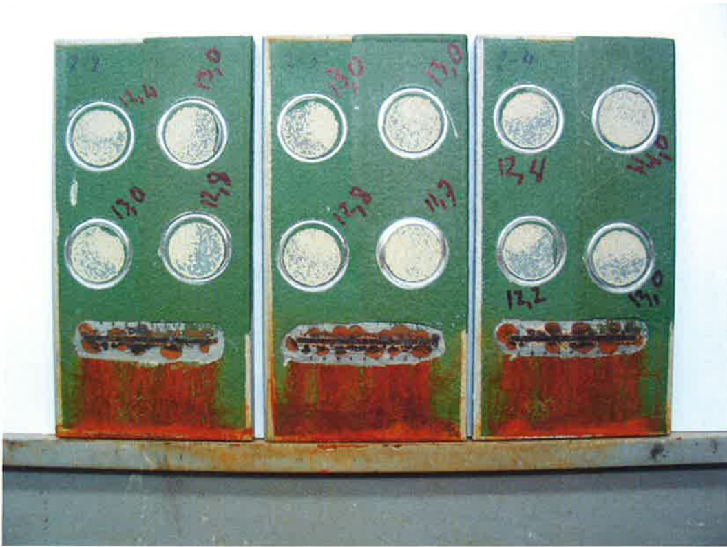
Photo 1. Cyclic ageing test, panels 2, 3 and 4.
